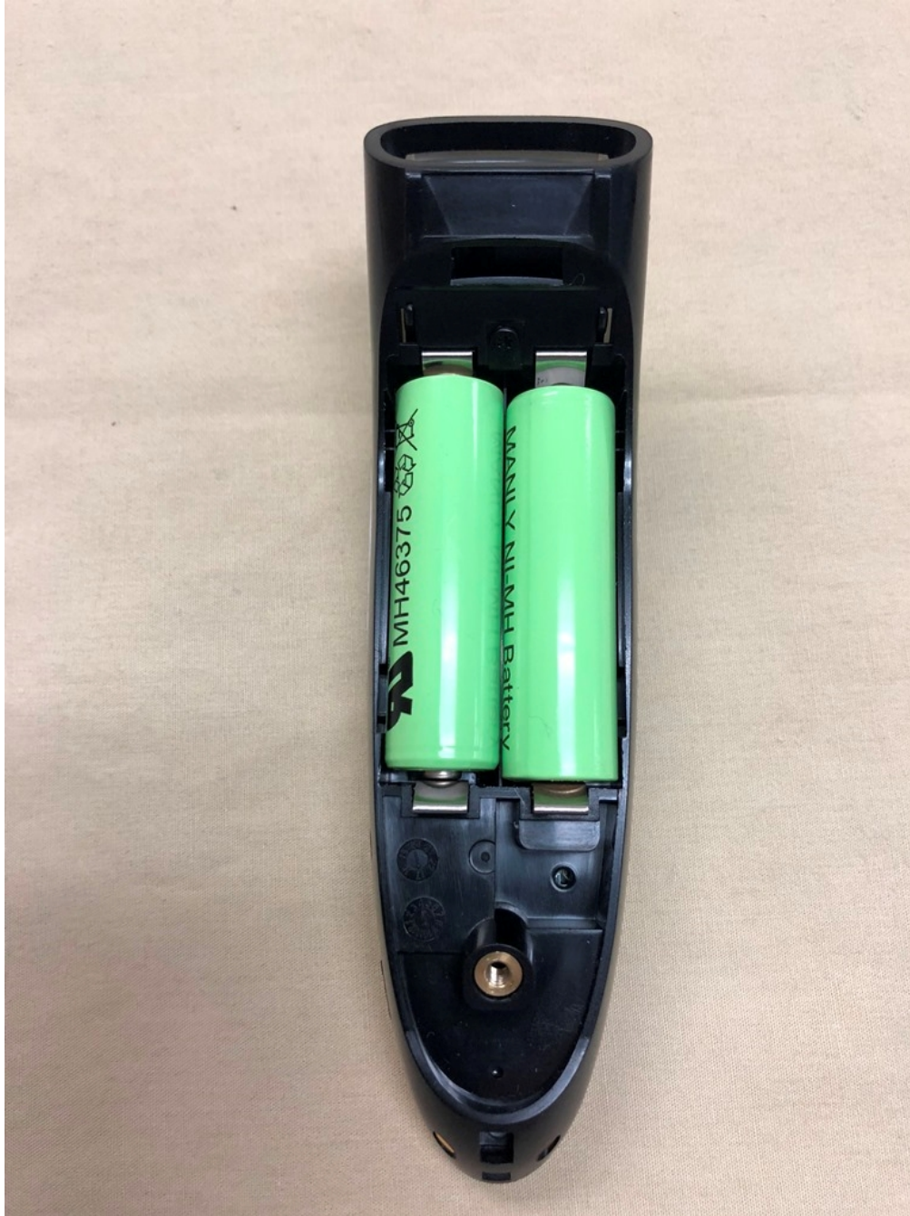
Figure 5 – S7xx Series – Rear Internal Showing Batteries
