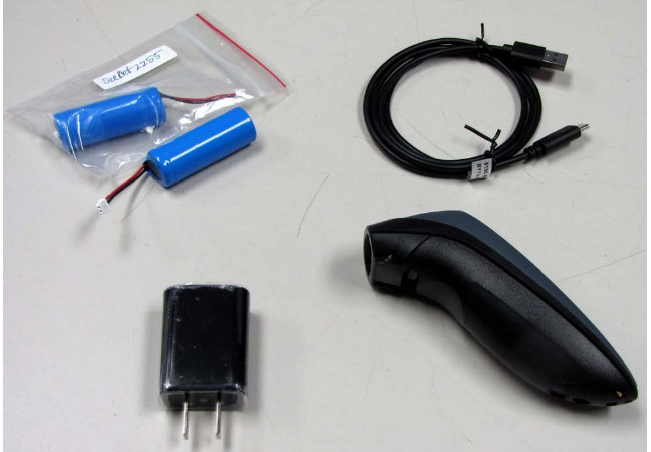
Figure 15 – D7xx Series - Overall View showing Battery, Optional Adapter and Cable
